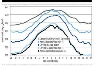
The graph shows wind resistance curves of two aerodynamic road bicycles compared to two light weight bikes with the same setup. In addition, a round-tubed frame (Canyon F8, 2010 model) with Mavic Cosmic Carbone wheels is shown as a reference and as a comparison to previous tests. The two Merida frames represent the extremes within the test field – no other pair measured further apart. Due to its slower wheelset, the reference frame has a flatter curve.
