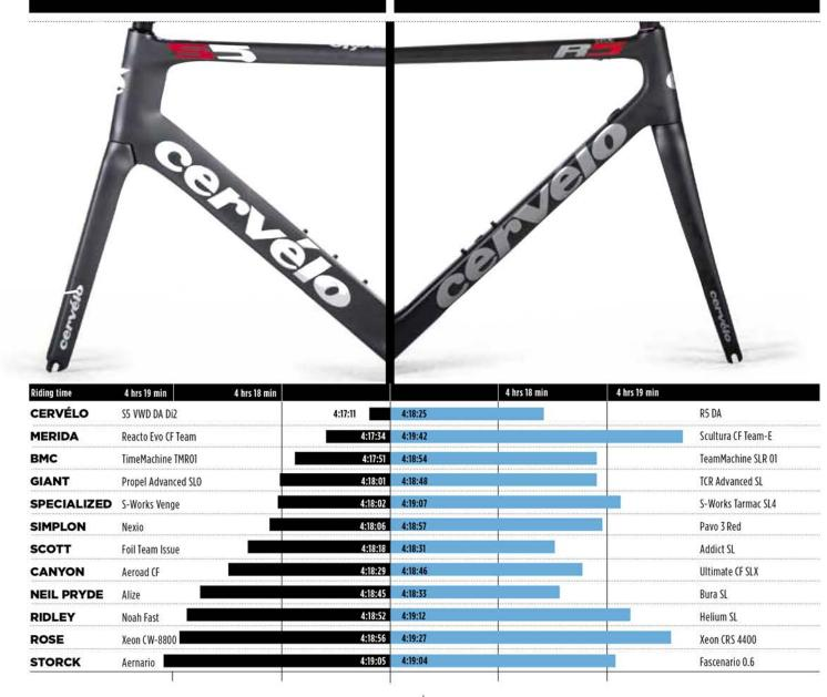
The bar graph shows the absolute ride times of the aerodynamic and lightweight bikes, paired by make and sorted according to the times of the aerodynamic road bikes. The shorter the bar, the faster the bike is on the simulated 100 km (62 mile) route with a total elevation gain of 2000 m (6562'). Under these conditions, the Cervélo S5 is the fastest bike with a ride time of 4 hours, 17 minutes and 11 seconds. The rider of the Merida Scultura
